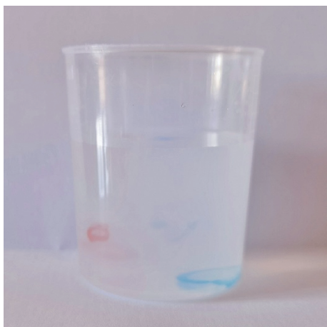
图3 苏丹红 III(左)和甲基蓝(右)在纳米乳液中扩散情况 Fig. 3 Diffusion of sudan III (left) and methyl blue (right) in nanoemulsion of EOPTN
