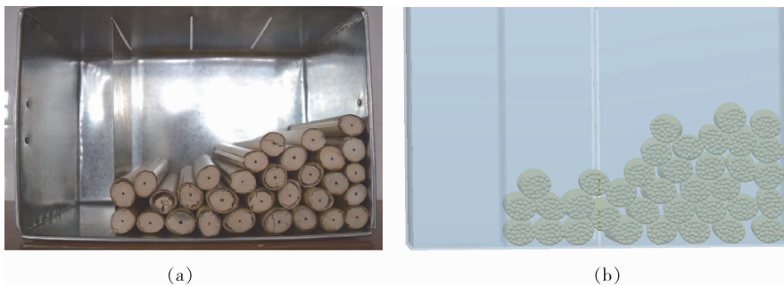
图 6 玉米秸秆堆积角验证试验结果 (a) 和对应的离散元仿真结果 (b) Fig. 6 Comparison between simulation results and experimental results
