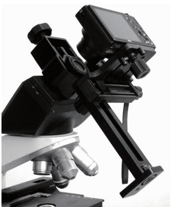
显示通过天文望远镜支架将普通数码相机连接到显微镜上。 A digital camera is connected to a microscope via an adapter.
