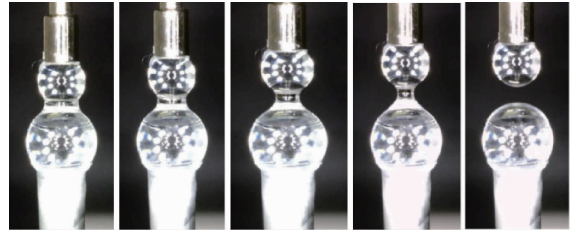
玻璃球径 d_1 = 2 \text{ mm} , d_2 = 3 \text{ mm} , # 100 硅油体积 V = 0.558 \mu\text{L} Glass beads d_1 = 2 \text{ mm} and d_2 = 3 \text{ mm} , # 100 silicon oil volume V = 0.558 \mu\text{L}
