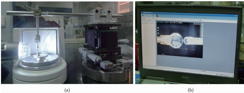
(a)左起:数字显微镜,天平称量盘及上下球, x-y-z 调位单元;From left: digital microscope, microbalance and glass bead samples, x-y-z stages;(b)笔记本电脑显示屏上经数字显微镜放大的上下球。Enlarged imagine of glass beads by microscope on PC monitor.
