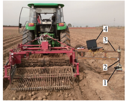
1. 摄像机; 2. 视角调节杆; 3. 支架; 4. 计算机 1. Camera; 2. Angle adjusting link; 3. Holder; 4. Computer
